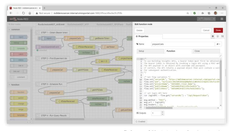
The first prepareCall function is used to configure the running and publishing of the schedule.
