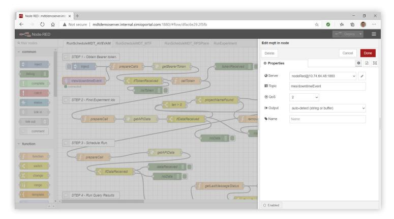
Then a Node-RED flow is deployed to capture the event from MQTT. Once captured, the schedule is rerun and published on Simio portal.
